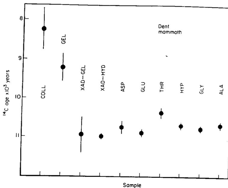
Figure 3. Dent mammoth AMS radiocarbon dates arranged in order of increasingly more pure chemical fractions. Abbreviations: COLL, collagen; GEL, gelatin; XAD-GEL, XAD-2-purified gelatin hydrolysate; XAD-HYD, XAD-2-purified collagen hydrolysate; ASP, aspartic acid; GLU, glutamic acid; THR, threonine; HYP, hydroxyproline; GLY, glycine; ALA, alanine. Error bars are 1 s.d. of the measurement from counting error.
